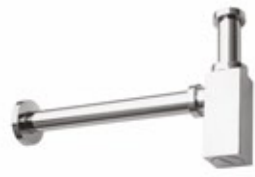
item code 1020 Bottle Trap (Zinc Body, Brass Nut) 32 mm with 300 mm long pipe
